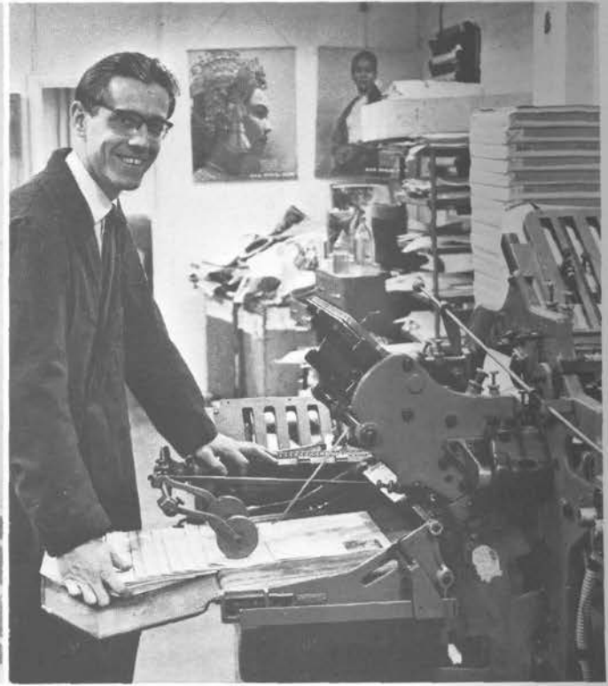
Literature is folded by this machine under the care of Peter London.
